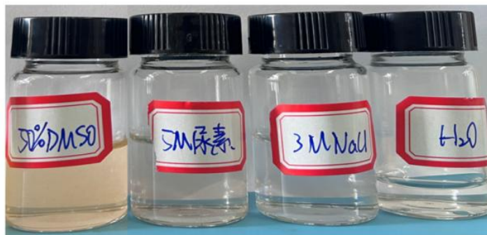
Fig. 3-7 Desorption of \gamma\text{-Fe}_2\text{O}_3 from PE pre-adsorbed nano- \gamma\text{-Fe}_2\text{O}_3
