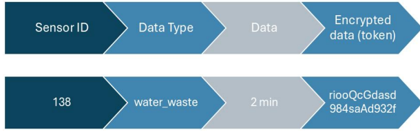
Figure 5. Schematic Representation of the Data Structure Sent from the Sensor to the Server, The first row shows the general format. The second row presents an example of the content.
