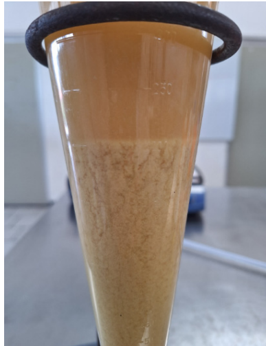
Figure 13. Sedimentation line in an Imhoff cone. Own photograph, 01/10/2025.
