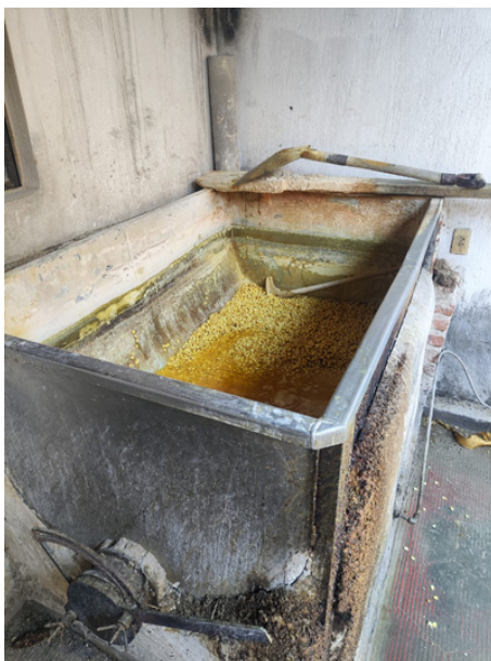
Figure 7. Nixtamalization kettle with nejayote recirculation. Own photograph, 01/15/2025.
