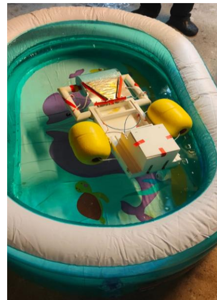
Image 3: Prototype Oil Skimmer in Action: Testing Oil Removal Efficiency in a Controlled Setup
