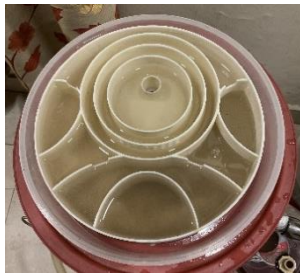
Figure 18: Top container with baffle filtration setup
