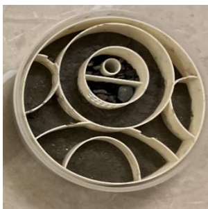
Figure 21: Third container with sand. An additional layer of fine aggregate was added in the circular chamber to prevent sand from passing through to the next container
