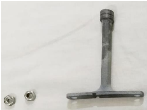
Figure 10: 3D printed components of pump holder
