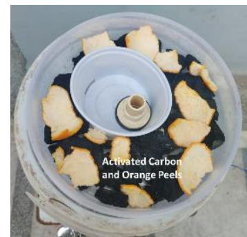
Figure 22: Fourth container with activated charcoal and orange peels
