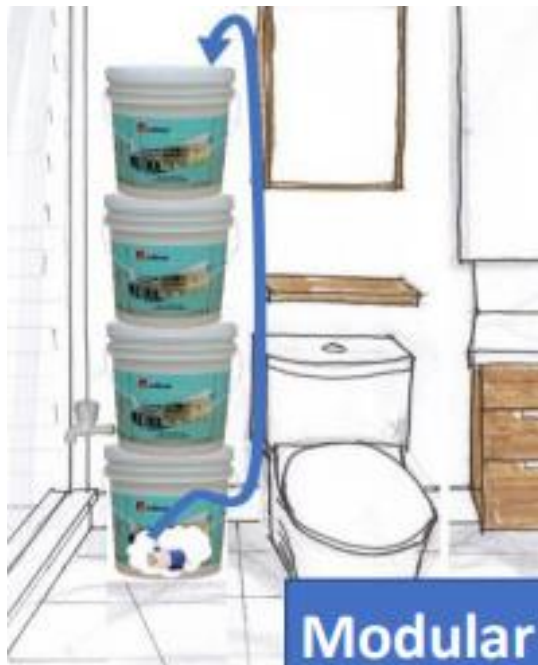
Figure 25: Modular setup of the BV where additional buckets can be added
