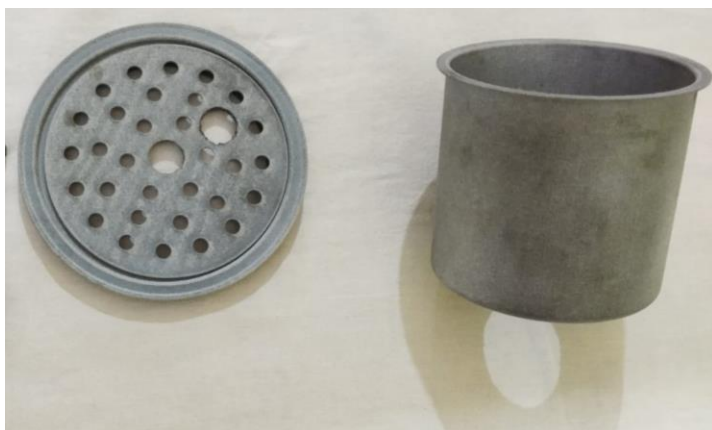
Figure 8: 3D printed components of the floor drain trap
