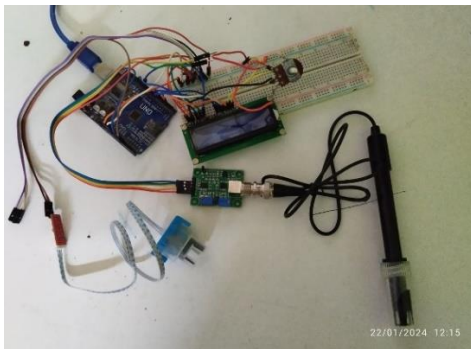
Figure 27: Arduino setup with LCD display, pH sensor and turbidity sensor
