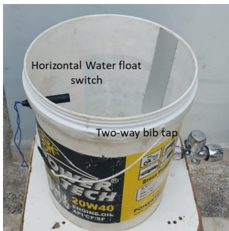
Figure 23: Middle bucket with water float switch and outlet
