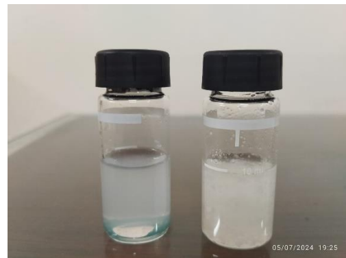
Figure 32 Inlet Grey Water Sample (Right); Treated Greywater Sample (left)
