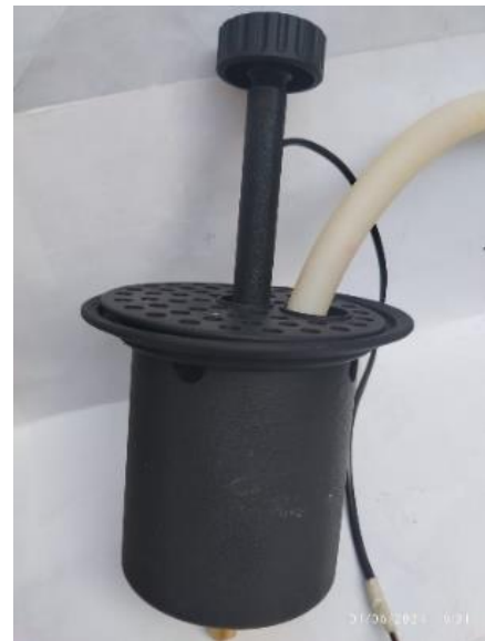
Figure 7: 3D printed Assembled Scupper Valve
