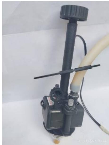
Figure 13: 3D printed pump holder
