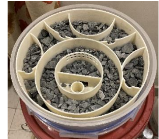
Figure 20: Second container with fine aggregate and baffle slabs
