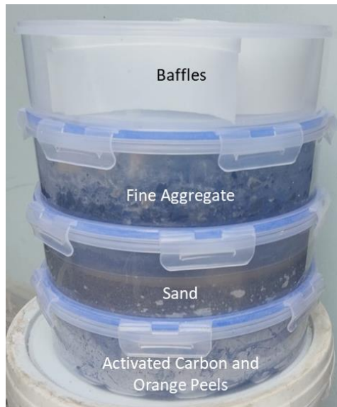
Figure 19: Four containers stacked together (housed in the top-most bucket)
