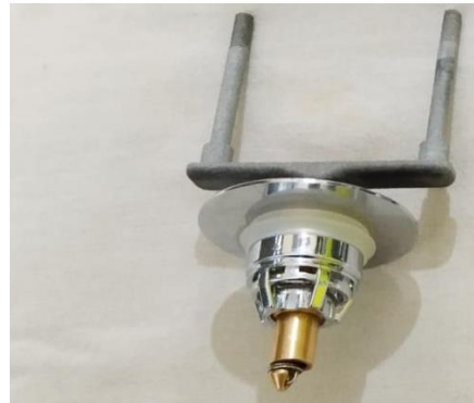
Figure 11: Pump Holder attached to the push-type drain stopper
