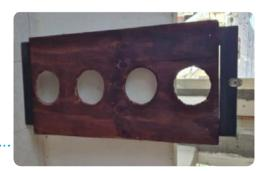
Figure 7. Wooden board with perforations to place the filters
