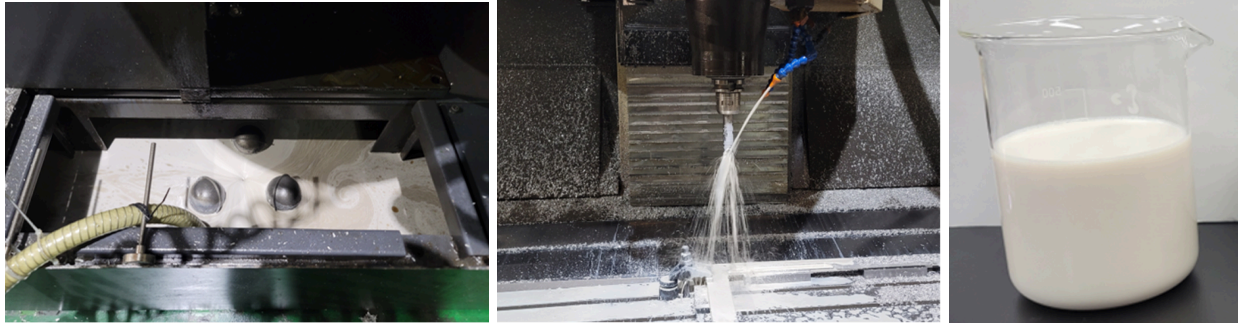
Figure 1. Demonstration of how water soluble cutting oil is used in metal cutting industries, including the cutting fluids tank (left), cutting fluids during metal cutting process (middle), and cutting fluids before the use (right).
