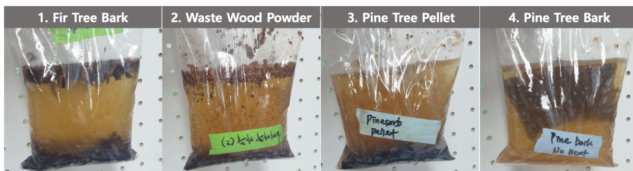
Figure 6. The demulsification effect of various tree types, including fir tree bark, waste wood powder, pine tree pellet, and pine tree bark (same amount of sulfuric acid added for all samples).
