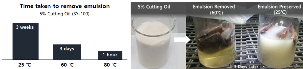
Figure 4. Amount of time consumed to separate the emulsion of cutting fluids for each temperature, including 25°C, 60°C, and 80 °C, organized in a graph (left) and photo (right).
