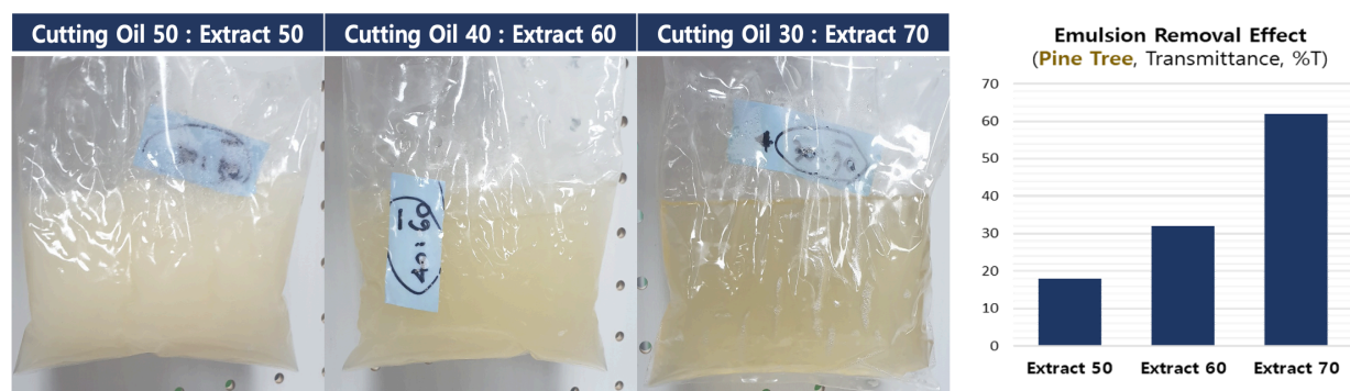
Figure 5. The effect of pine tree extract in separating the emulsion of cutting oils, illustrated in a photo (left) and graph (right). Pine tree extract and cutting oil have three different ratios, - “extract 60” on the graph signifies that 60% of the solution is pine tree extract and remaining 40% is cutting fluids.
