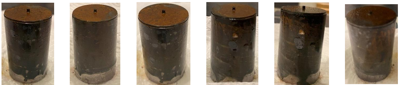
Figure 4: Images of Biofilm Growth on Stainless-Steel with CO Coating
