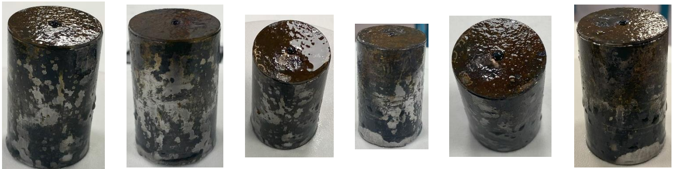
Figure 3: Images of Biofilm Growth on Stainless-Steel with CinO Coating
