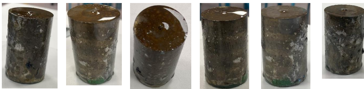
Figure 5: Images of Biofilm Growth on Stainless-Steel with TTO Coating
