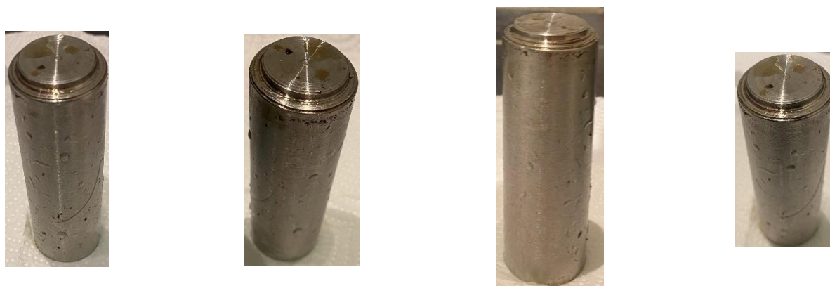
Figure 6: Images of Biofilm Growth on Stainless-Steel with Chemical Agent Coating
