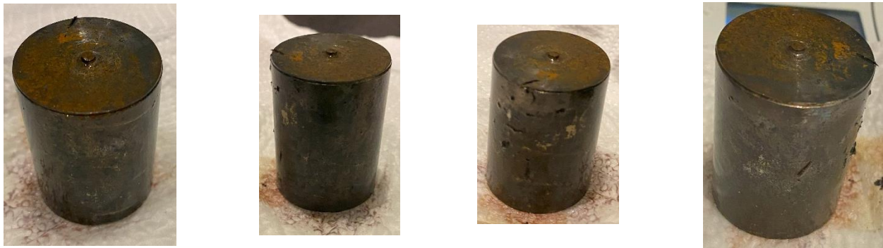
Figure 2: Images of Biofilm Growth on Stainless-Steel with No Coating (Control group)
