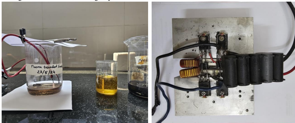
Figure 7: High Voltage Plasma process and working method & Plasma generator circuit
