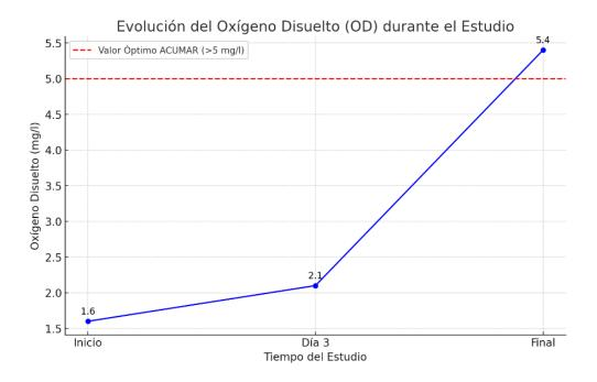
Graph showing improvement in dissolved oxygen levels from the beginning to the end of the study, indicating effective photosynthesis by the microalgae.
