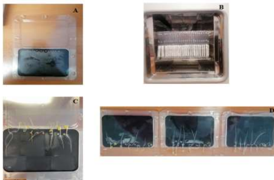
Fig. 1. Pictures of the Phytotoxkit Microbiotest plant growth during the experiment. (A shows the seed germination process during day 1 of the experiment, B shows the incubation of the test plates in the incubator at 25 °C and C and D show how the roots and shoots of the plants grow)
