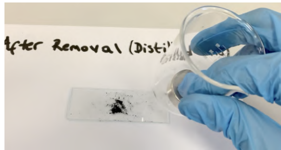
Figure 23: M-CNTs are being separated from MPs after the removal process to be recovered
