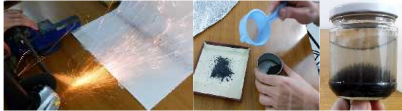
Fig.24: obtaining iron particles, separating the smallest particles, washing the particles
