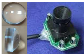
Fig. 9: m12 optics, inverted lens webcam
