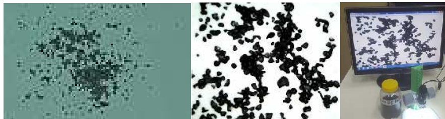
Fig. 28: iron powder various granulometries
