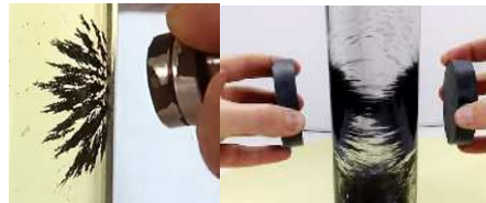
Fig. 20: homemade ferrofluid in oleic acid and with alcohol
