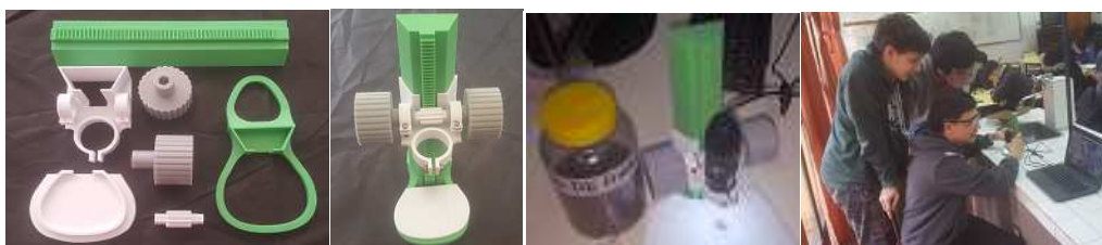
Fig. 11: 3D printed parts, assembly of parts, assembled microscope, students using it
