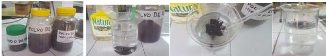
Fig. 25: different granulometries of iron powder, decantation according to its granulometry, finer iron powder
