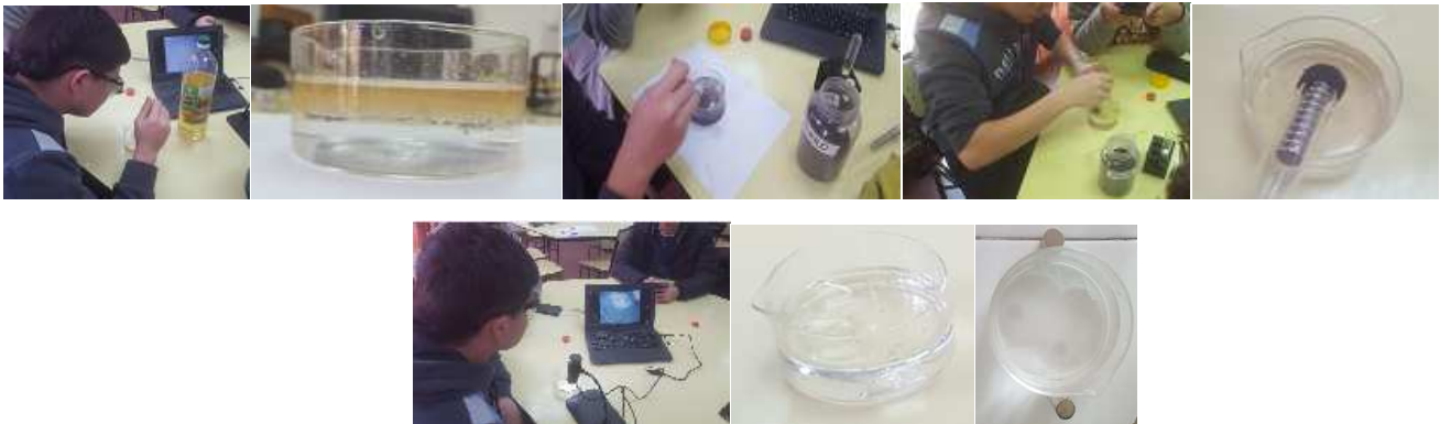
Fig. 13: microplastics and oil, placing iron powder and mixing, passing magnets, observing under a microscope, partial result, final result
