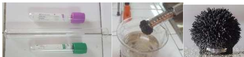
Fig. 26: Plastic tubes and glass test tube, stirring ferrofluid, magnetic power of neodymium magnets
