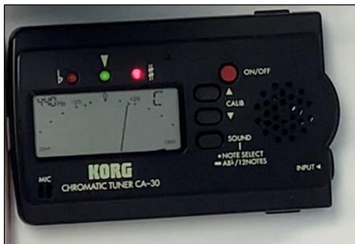
Figure 11. Tuner displaying the frequency value and its variation in the measurement of the positive control with stones from Olloki. Source: Own elaboration.
