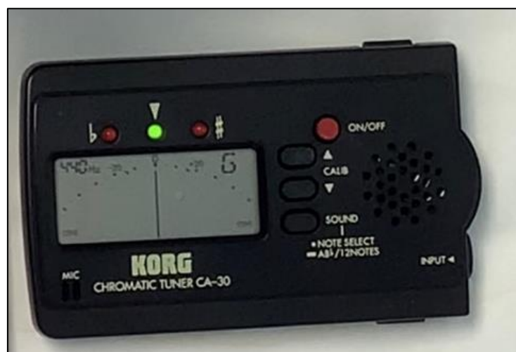
Figure 7. Tuner displaying the frequency value and its variation in the measurement of the positive control with the metal bottle. Source: Own elaboration.
