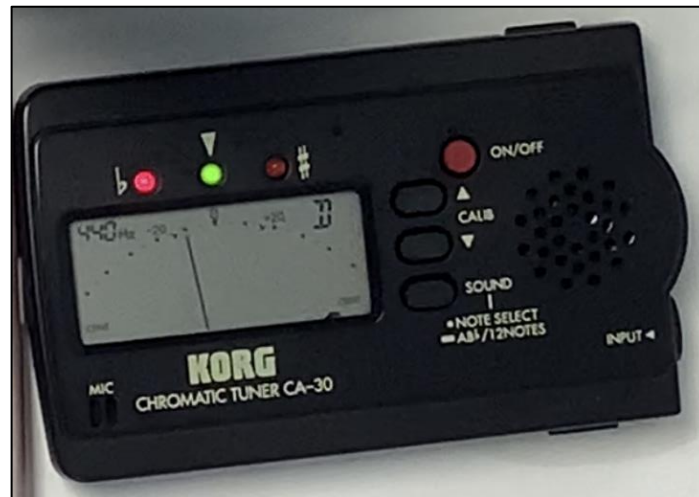
Figure 12. Tuner displaying the frequency value and its variation in the measurement of the sample from Olloki. Source: Own elaboration.
