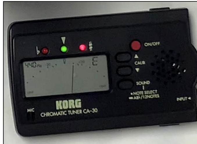
Figure 15. Tuner displaying the frequency value and its variation in the measurement of the sample from Ororbia. Source: Own elaboration.
