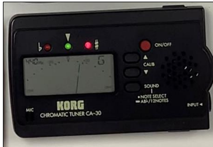
Figure 6. Tuner displaying the frequency value and its variation in the measurement of the positive control with microplastics. Source: Own elaboration.
