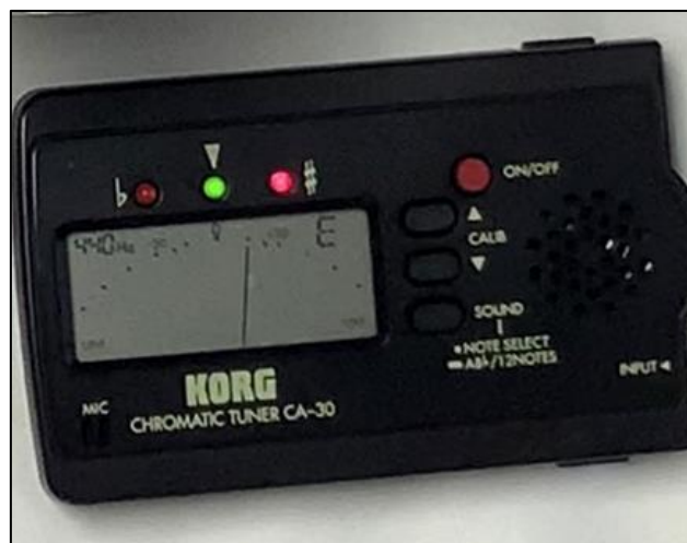
Figure 14. Tuner displaying the frequency value and its variation in the measurement of the sample from Ororbia. Source: Own elaboration.
