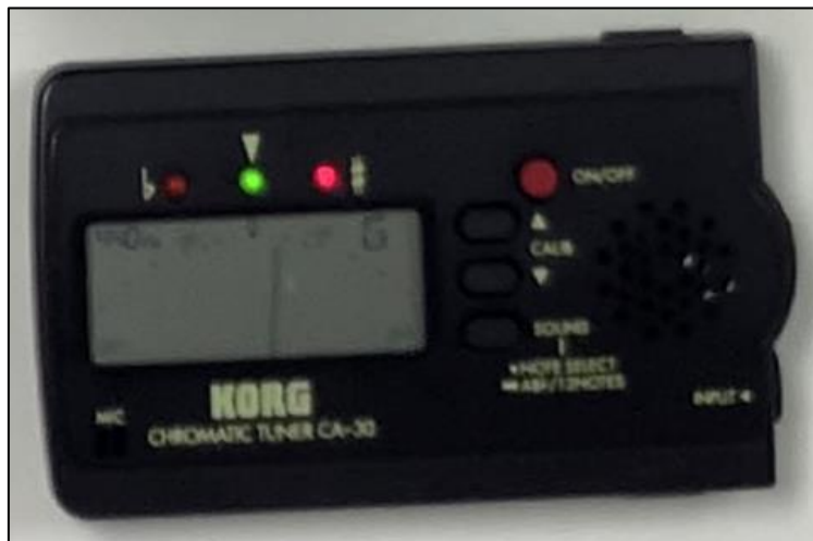
Figure 5. Tuner displaying the frequency value and its variation in the measurement of the positive control with macroplastics. Source: Own elaboration.
