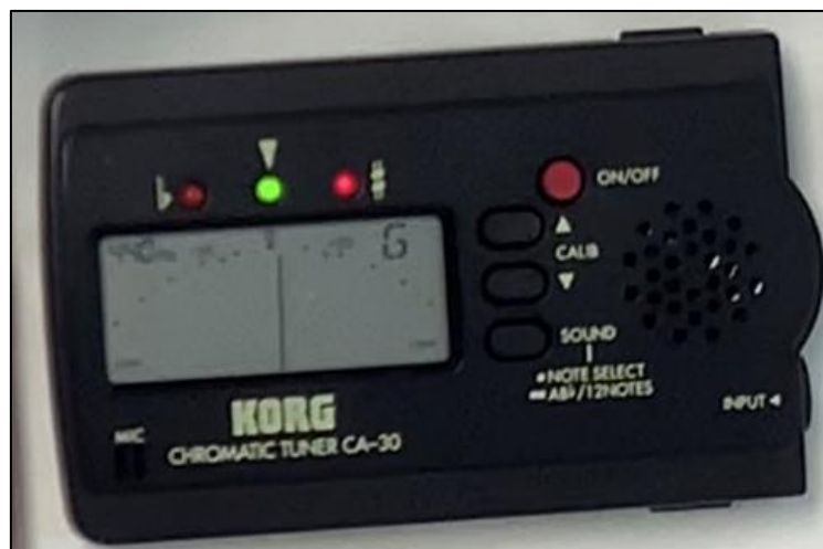
Figure 8. Tuner displaying the frequency value and its variation in the measurement of the positive control with the salinity concentration. Source: Own elaboration.
