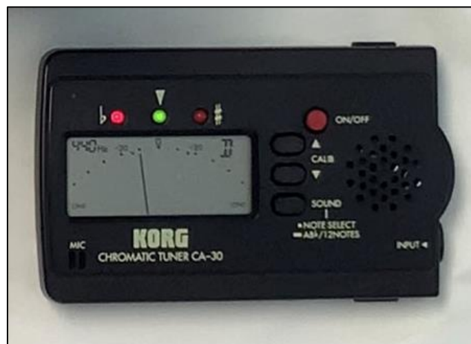
Figure 13. Tuner displaying the frequency value and its variation in the measurement of the sample from Club Natación. Source: Own elaboration.
