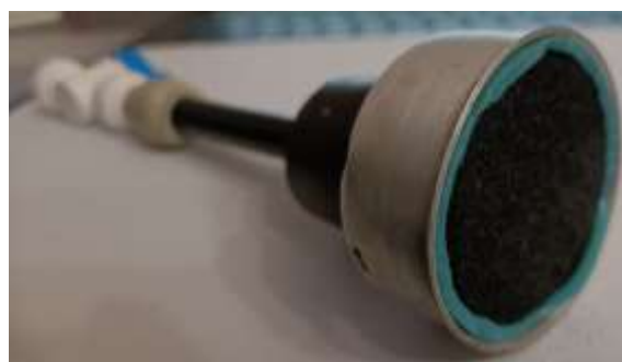
Figure 2.2 – The nozzle of the device for water purification
