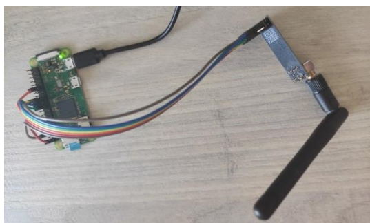
Figure 17: Raspberry Pi and nRF Module in Communication System
