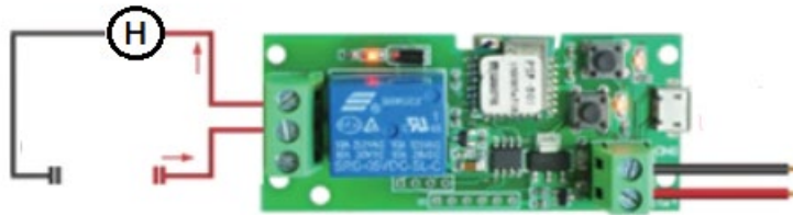
Fig.8 Diagrams for connecting remote modules to a controlled circuit
