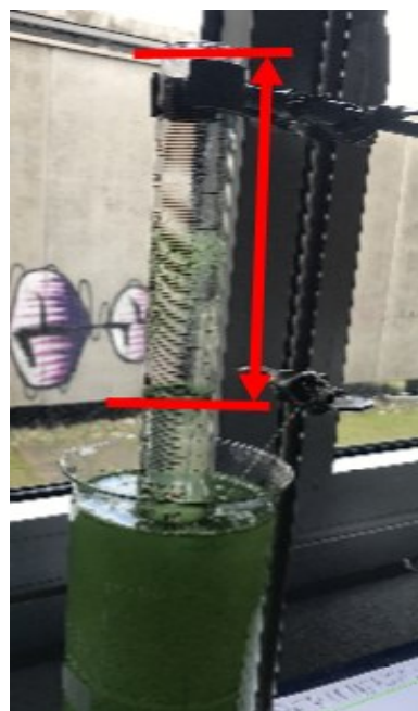
The red lines help visualise the lowering of the culture level in the cylinder due to the production of dioxygen.
