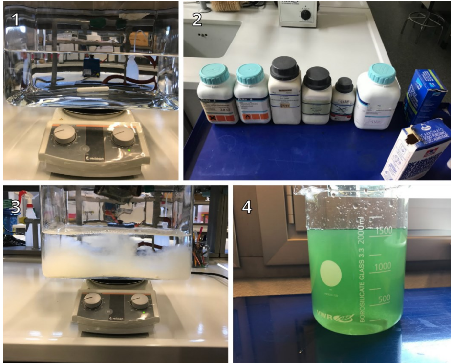
1. Deionised water in the aquarium above the magnetic stirrer before adding the salts. 2. Salts used. 3. Aquarium with deionised water placed on top of the magnetic stirrer immediately after the addition of the salts. 4. Becker containing the first culture started with Zarrouk's medium.
