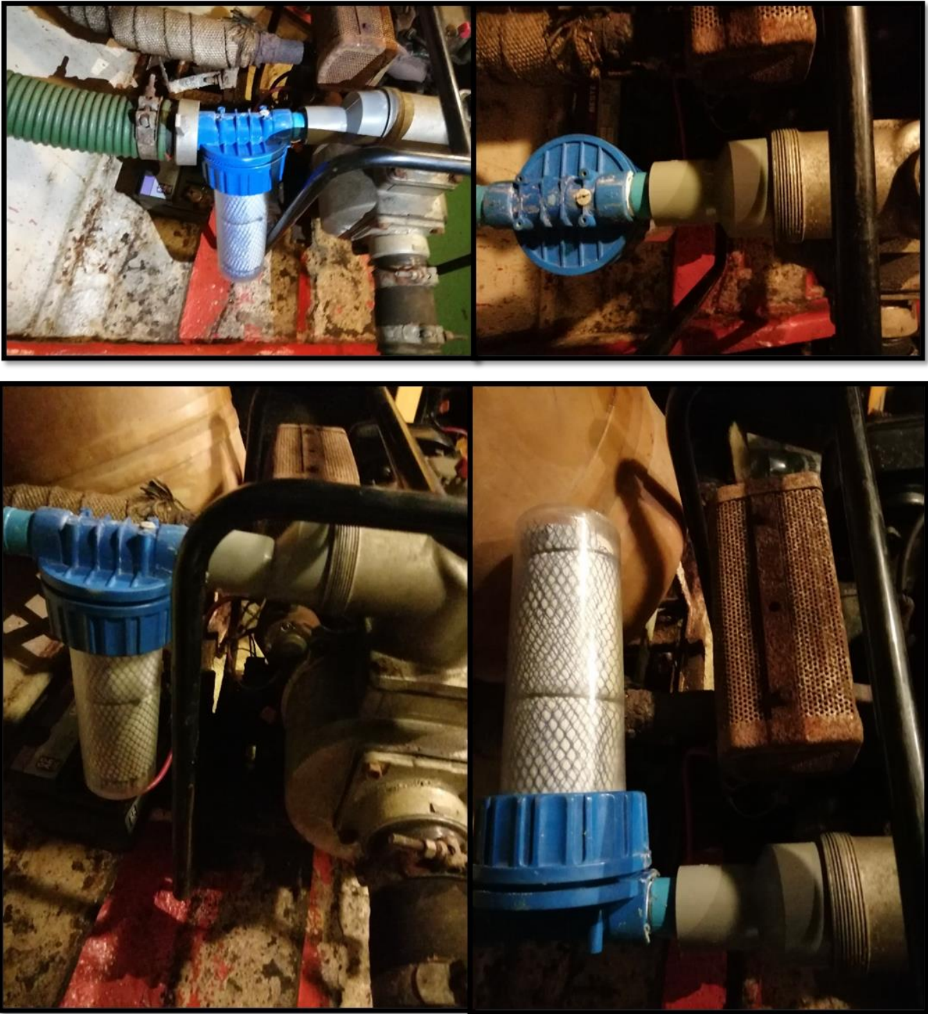
Image N°8 Posture of human hair filters (F.C.H.) at the outlet of the "Bilge" pump
