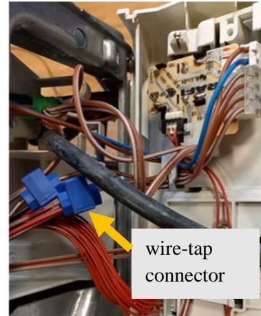
Figure 16 - shows the tapping of the cables with on/off cables with wire-tap connectors; photo: Luise Mast.
