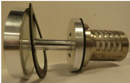
Figure 28 - shows the complete filter unit assembled (lint filter with microplastic filter); Photo: Luise Mast.
