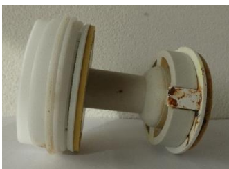
Figure 9 - Fig.9a (left) - shows current lint filter Miele, Fig. 9b (middle) shows new lint filter for Miele and Fig.9c (right) shows new lint filter for Bosch; photo/drawings: Luise Mast.
