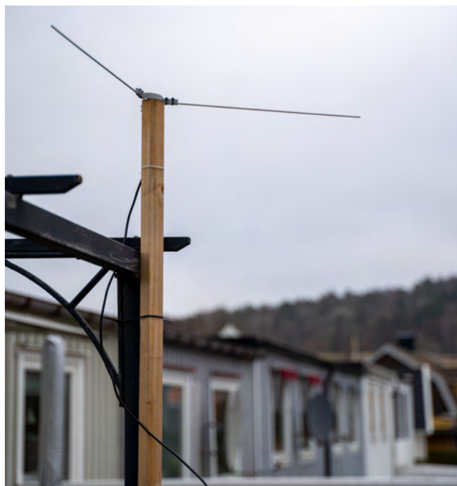
Figure 4: Assembled antenna construction, secured with cable ties on a balcony.
