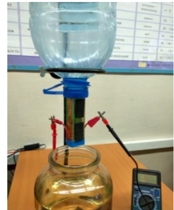
Fig.5. A model MHD generator
