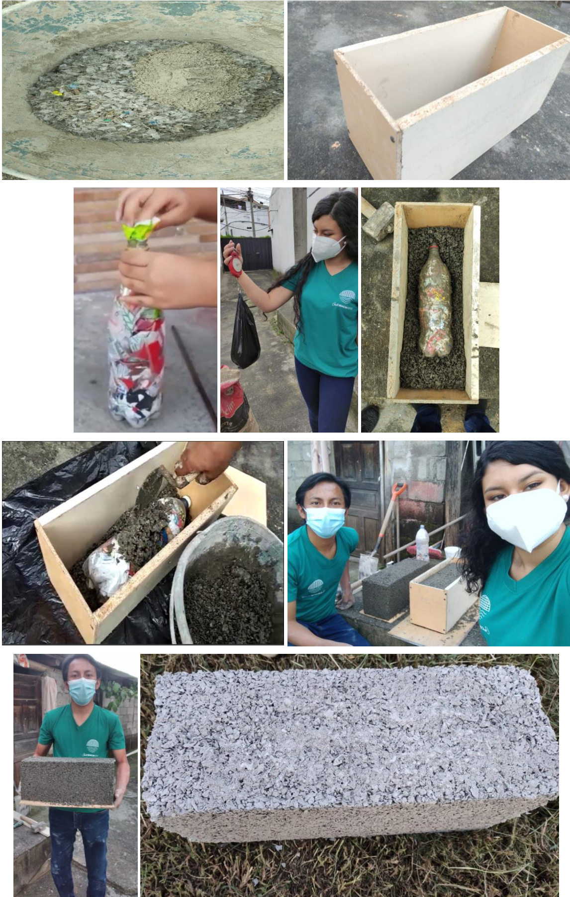
Illustration 8 Eco-block elaboration process
