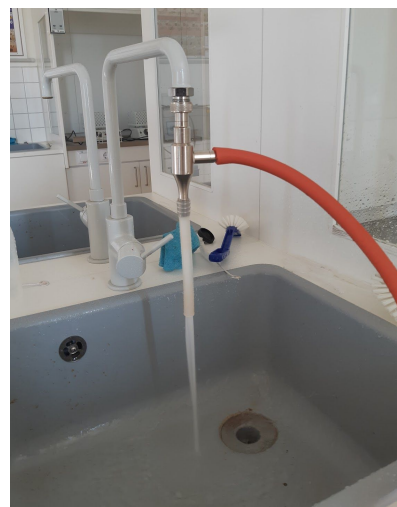
Figure 6: Assembled equipment for filtration with suction. (Source: own picture)
