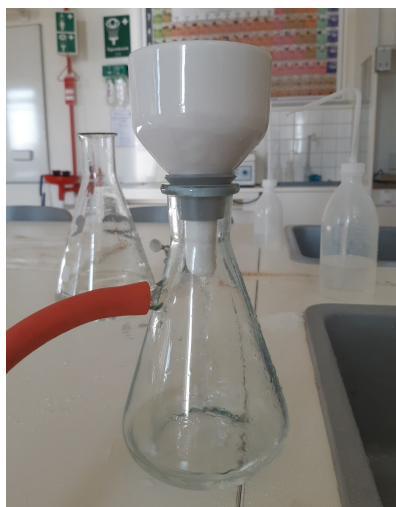
Figure 5: Assembled equipment for filtration with suction. (Source: own picture)
