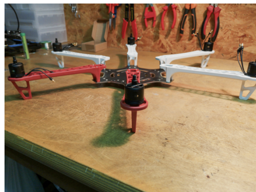
Figure 2: assembling the frame, arms and motors of the drone
