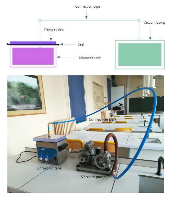
We connected our vacuum pump to an ultrasound tank. To do this, we had to build a plexiglass lid 3 centimeters thick. The ultrasounds were on at the same time as the pump and that is how we could bind our two ideas. For the rest, the precedent protocol was applied all the same.
