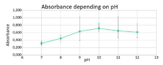
Results on this graphic show an optimum at pH 10. Indeed, from pH 7 to pH 10, absorbance grows to 0.717. At a higher pH, results are lower, so it seems that a pH 10 solution would be optimal for our washing protocol.
