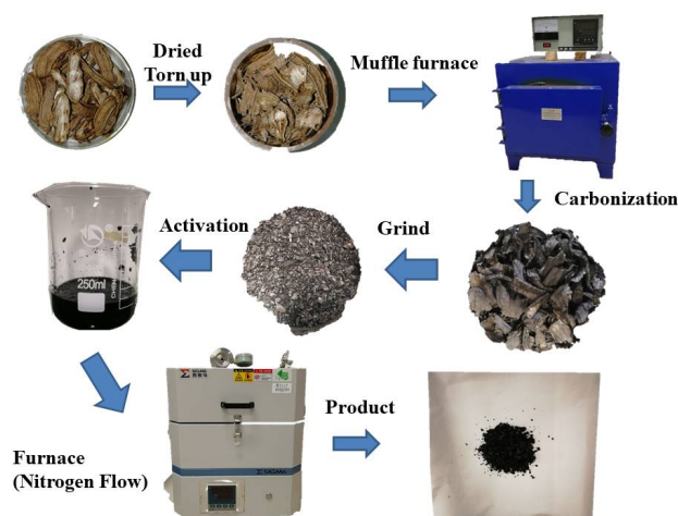
Fig.3. The preparation process of peanut shell based activated carbon
