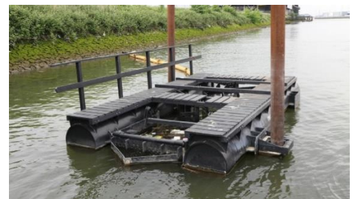
Figure 2 - One of the plastic litter traps from Recycled Island Foundation (Recycled Island Foundation, 2018)
