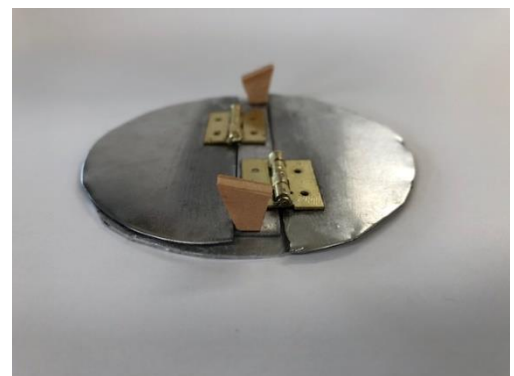
Figure 14- Side view metal heart valve (closed)
