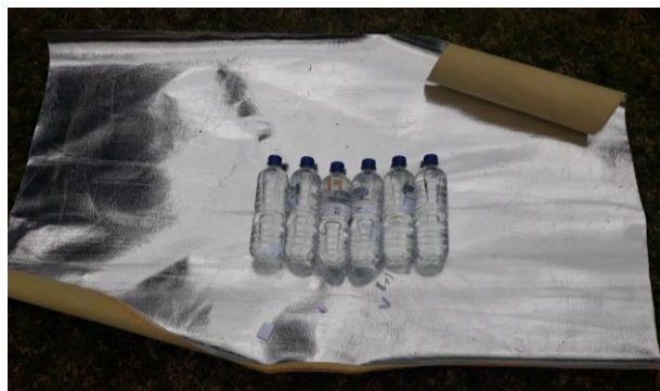
Figure 13: Bottles of water prepared for SODIS solar UV exposure with SODIS Stickers in place in front of and behind the water.
