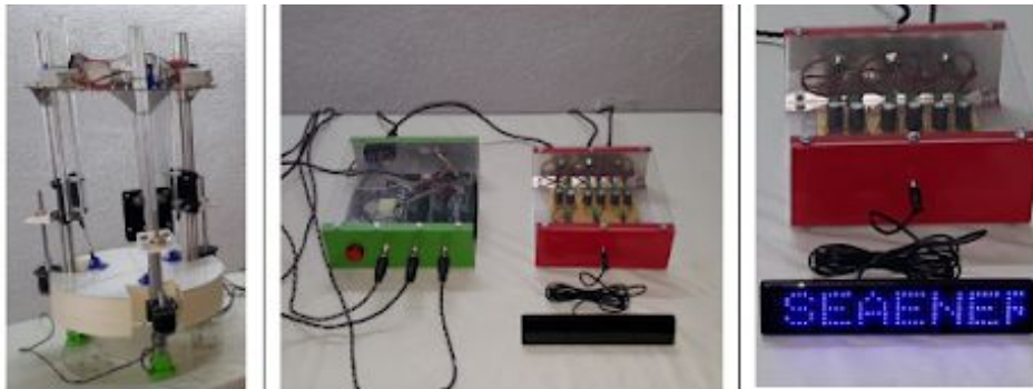
Figure 43. Overview of the finished prototype, with the buoy and the delta structure (left), the wave simulator and the power generator (center), and the display working (right).
