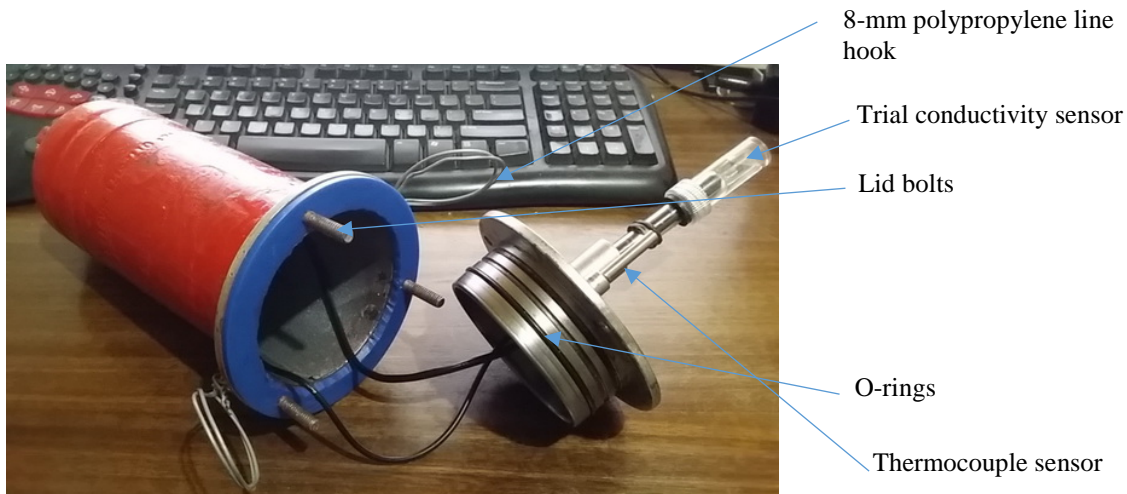
Figure 4. Tester probe prototype 1 showing sensors and waterproofing system details.
