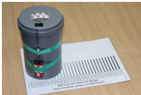
Fig. 5. A device for assessing turbidity (transparency) and water color. The camera Canon and the Photoshop program were also used to evaluate the color of the water.
