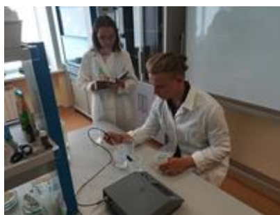
Fig. 3. Conducting measurements of the concentration of water components using I-160 ionomer.
