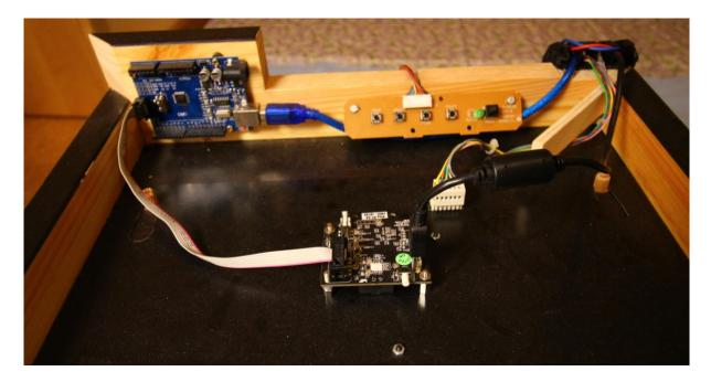
The camera has its own microprocessor (NXP LPC4330) for image processing. This communicates via SPI with an Arduino (AT MEGA 328P). The Arduino then passes the data filtered and sorted per serial interface (via USB) to the connected PC.
