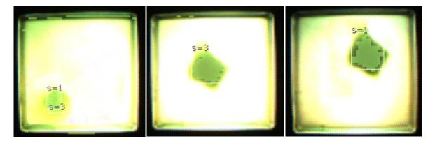
The illustration shows that the video processing has identified the colonies of algae. Different signatures indicate the detected relative density of organisms.
