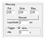
Measurements are processed every 5 seconds. For that a uniform bright white light is displayed for 2 milliseconds.
