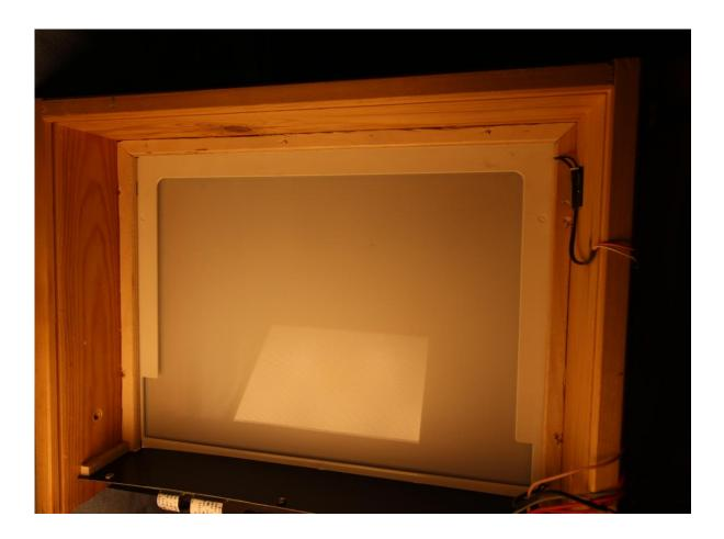
Under the LCD screen there is a diffuser whose task is to distribute the light coming from the light source as uniformly as possible on the LCD.
