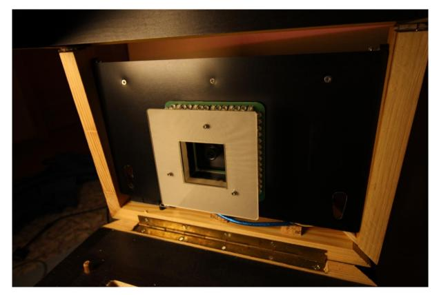
The light arranged around the camera allows the regeneration of the algae. This light ensures optimal conditions for photosynthesis between experiments and helps to prevent the Chlamys from being exhausted and becoming sluggish.
