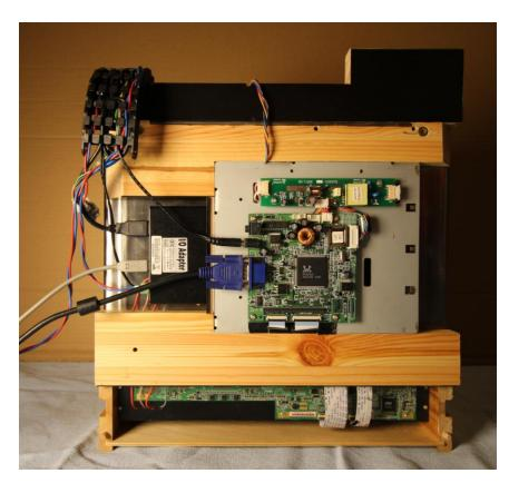
The LCD can be controlled via a VGA interface.
