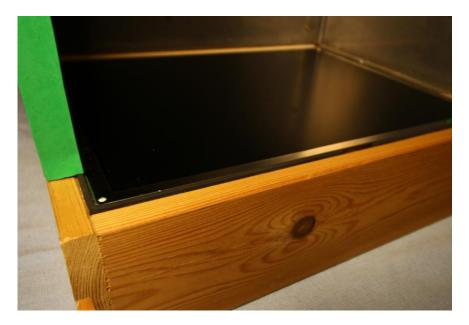
In order to be able to vary the intensity and colour of the light impinging on the algae pixel by pixel, there is an LCD (Liquid Crystal Display) in front of the light source. The algae are then supposed to swim above the light source. The used TFT-LCD has 1200 x 800 pixels which can display the colors red, green and blue in different intensities, the refresh rate is 30 fps.
