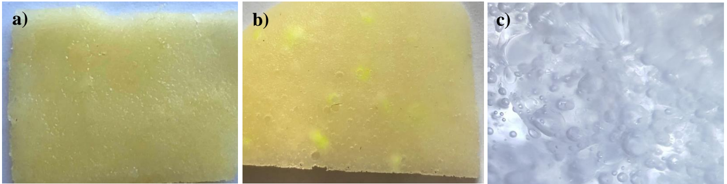
Figure 6. Sample image of the sample-retaining bioplastic after exposure to: a) water samples without Pb^{2+} and Ni^{2+} , b) water samples containing Pb^{2+} and Ni^{2+} and c) an image of the 2017 bioplastic sample developed by Nithiyanandam [6].
