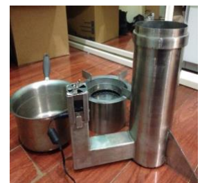
Photo 7: a biochar gasifier in which the heat energy produced upon pyrolysis can be used for household cooking purposes (components include a fan, crown, reactor body,
