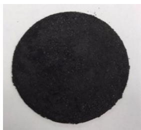
Figure 9: rGO-coated MCE filter
