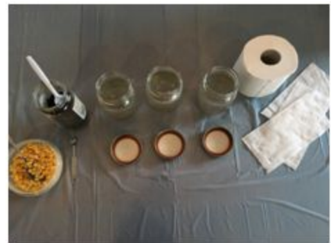
Figure 2 Three trials of each sample were prepared and kept out of sunlight for seven days, agitating for five seconds every 24 hours.
