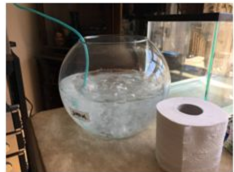
Figure 3 Three trials of toilet paper sample in sewer simulation test for three hours of ‘lazy river’ agitation.
