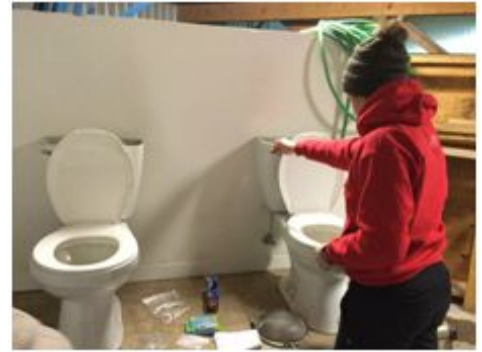
Figure 4 Three trials of each sample were flushed down the low flow toilet and same parameters were repeated for the regular flow toilet as well.
